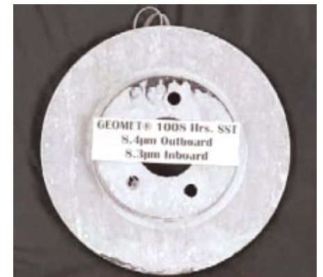
Only the braking surface is considered significant for evaluation in this test
