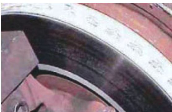
Inboard surface of GEOMET® coated rotor in dynamometer test after the first five instrument check stops.
