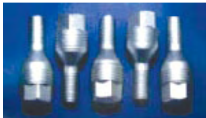
GEOMET® L 10 cycles of APGE. Uncoated internal threads were waxed before testing.
