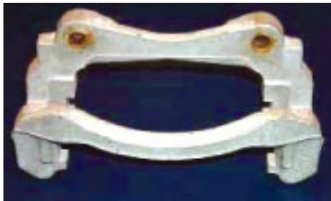
GEOMET® L 10 cycles of APGE. Uncoated internal threads were waxed before testing.
